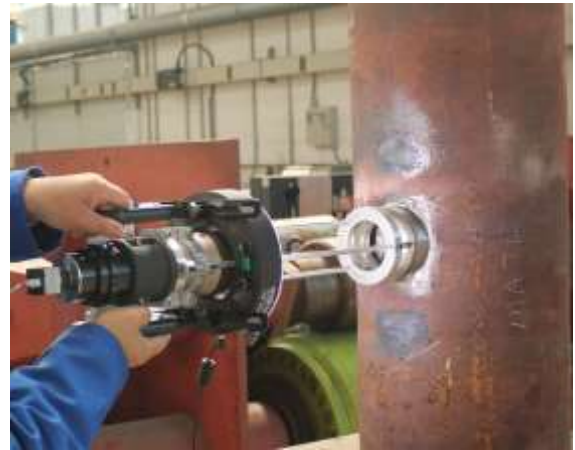
Rapid CreepImage inspection performed using a camera positioning jig.
