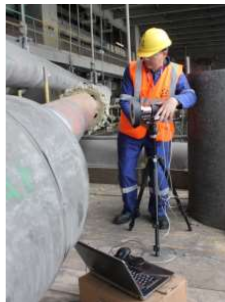
Assessment of CreepImage repeatability and reliability performed on a high temperature steam pipe during a power plant outage.
